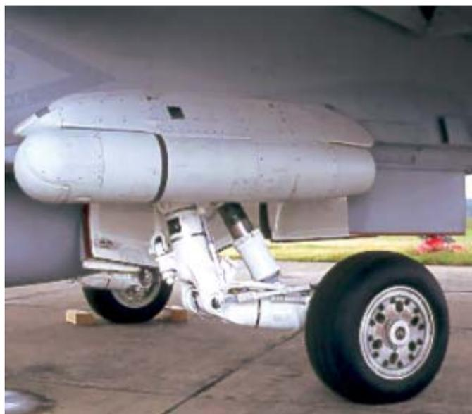
Fig. 7 - Forward Looking Infra Red – Flir (13)
